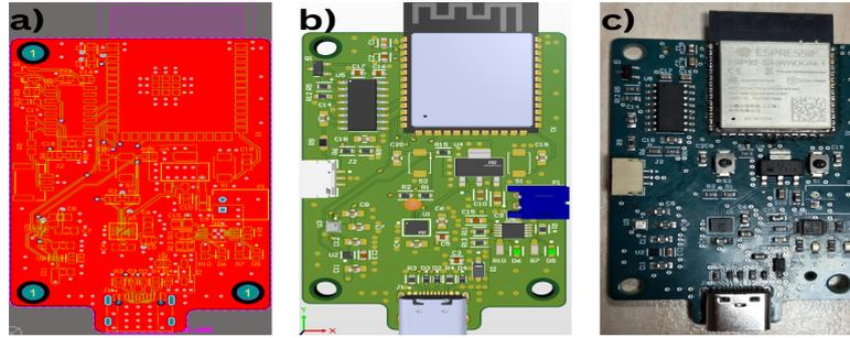
(A) a) 2D footprint of the designed PCB on Altium b) 3D view of the design c) Mounted PCB after fabrication.
