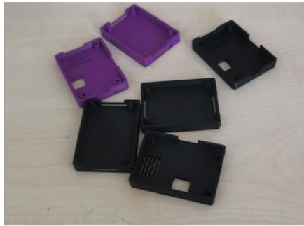
(B) 3D printed cases for the PCBs for mechanical safety of the PCBs.
