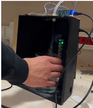
Figure 4A: Glass detected, filling continues
