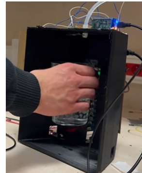
Figure 4B: Glass not detected, filling stopped
