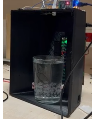
Figure 5B: Glass detected, enough water, filling stopped with a small error
