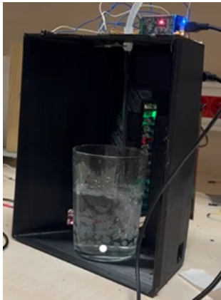
Figure 5A: Glass detected, not enough water, filling continues
